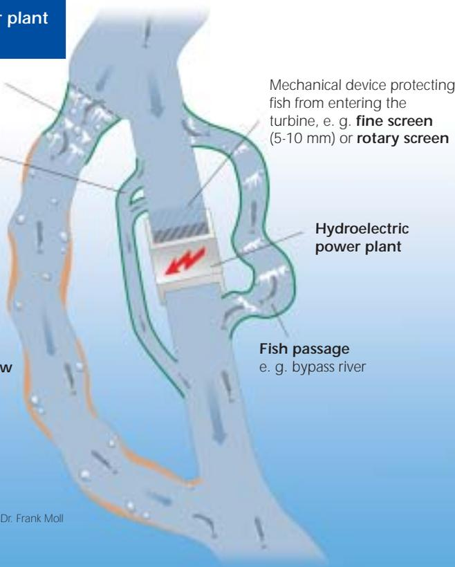
Mechanical device protecting fish from entering the turbine, e. g. **fine screen** (5-10 mm) or **rotary screen**
