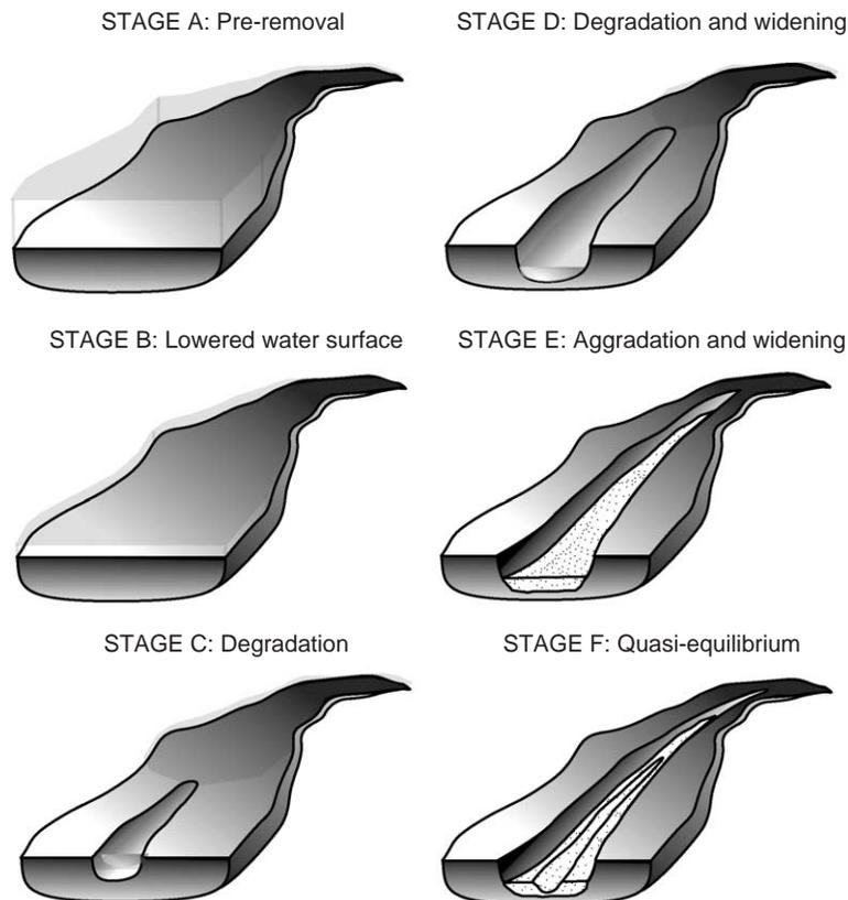
Fig. 1. Conceptual model of channel changes through time in reservoir following removal of a small dam (adapted from Doyle et al., 2003a).
